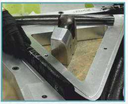
Bladder moulding is a popular manufacturing process used in the production of high-performance carbon fiber composite parts. It is an ideal process for producing parts with complex shapes and high-quality surface finishes which are not possible with conventional manufacturing method. We have inhouse capability to make moulds for vacuum moulding for different shape products.
