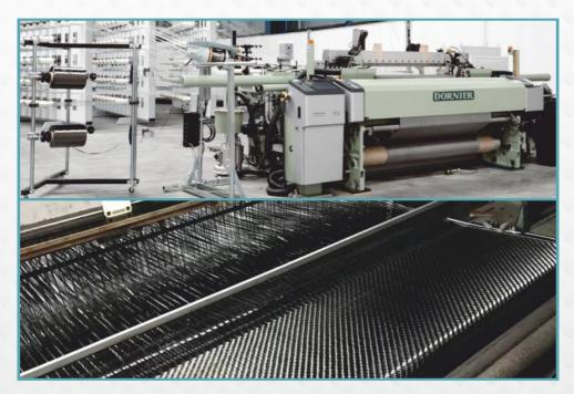
We use Dornier Rapier Weaving Machine P2 which is the latest state-of-theart machine from Lindauer Dornier GmbH, Germany to weave carbon, aramid, basalt or glass fiber fabric for multiple applications. These include reinforcement in civil engineering and construction applications, for hand layup for different kind of parts used in aerospace, automobiles, etc, for making BD prepreg for moulding & other applications, etc.
